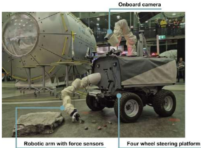
Figure 2: Interact rover (four-wheel-steering) and setup for manipulation and driving operation with sigma.7 during preliminary tests of the integrated system.
