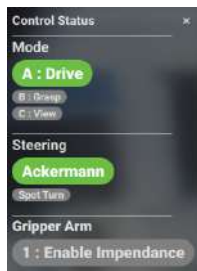
Figure 5: Highlight of the control status panel: visual confirmation of the operation mode (drive, grasp or view)
