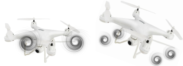
Fig. 1. Illustration of blade tip vortices at different flight conditions. The figure to the left corresponds to the rotorcraft being in OGE (Out of the Ground Effect) hover; the figure to right, forward flight.
