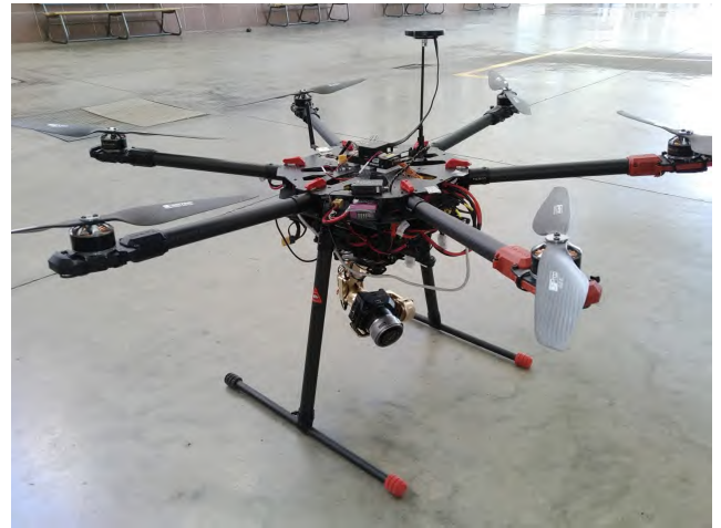
FIGURE 7. One of the drones used during our field experiments, with the cinematographic camera mounted on the gimbal.
