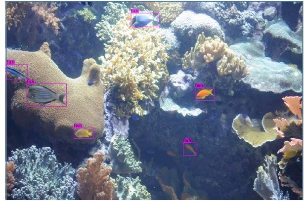
Fig. 4. The bounding boxes (in pink) predicted by YOLO detector.
