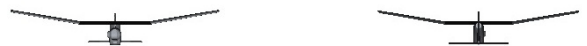
Fig. 2: The UAV under symmetrical rotations. While the UAV on the left image moves towards the camera, the UAV on the right image moves away from the camera.
