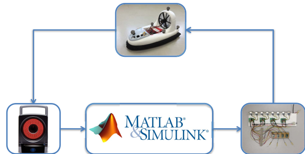
Fig. 10. Hovercraft integrated measurement and command architecture.
