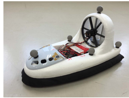
Fig. 9. Hovercraft with batteries, radio receiver, and motion capture markers.
