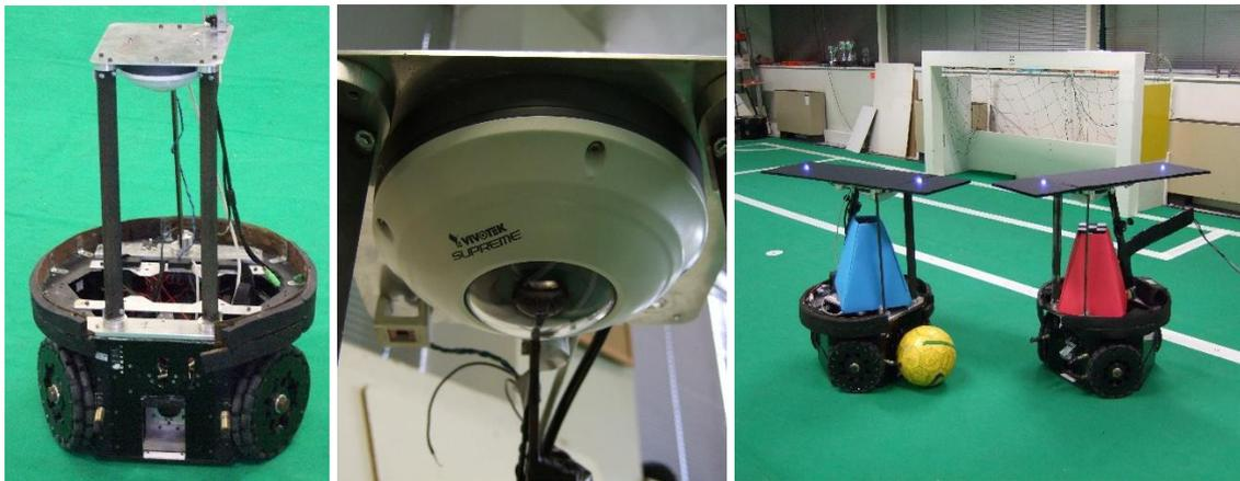
**Figure 1.1: From left to right: MSL robot; Omni-directional camera detail; MSL robots in the laboratory test field, with ground-truth markers installed.**
