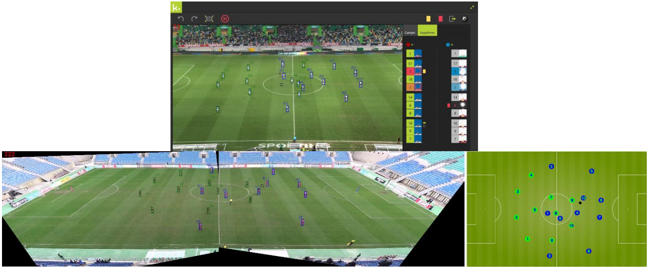
Figure 1. Top, web interface for the Tracking Editor with an image showing the results from a single camera. Bottom left, results of the ball and players detection and assignment to their respective team (two cameras). Bottom right, the representation of the real player's position in the pitch for the image on the left.
