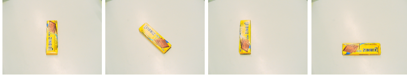
Fig. 2. The four different poses used for our experiment, demonstrated for Cookies . The left-most image shows the object in the standard pose used for training. The remaining three views show the object in different orientations and positions.
