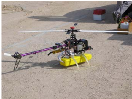
The Vario Xtreme Helicopter equipped with control electronics. Left: Helicopter ready to takeoff; Right: Detail of the control electronics and motion sensors.
