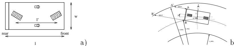
Figure 1: a) Schematic representation of a rhombic vehicle, showing its main dimensions; b) Vehicle alignment errors and clearance space ( space = \min\{\overline{AA'}, \overline{BB'}\} ) in the TB gallery.
