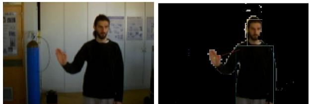
Fig. 6. Vision system. Left: original image. Right: background segmentation with human (the frame corresponds to the template matching) and hand detection.
