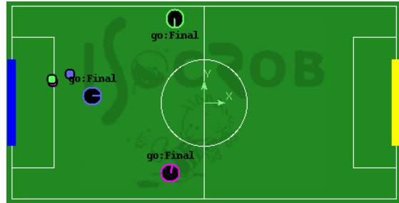
Fig. 8 – Bottom robot receives ball position from top robot, while top and leftmost robot disagree.
