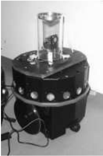
Figure 1: Catadioptric system assembled on the robot.
