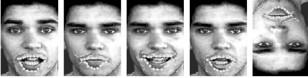
Fig. 17. Extracted edges on five of the 20 test images. Matched edges are marked with bigger dots.
