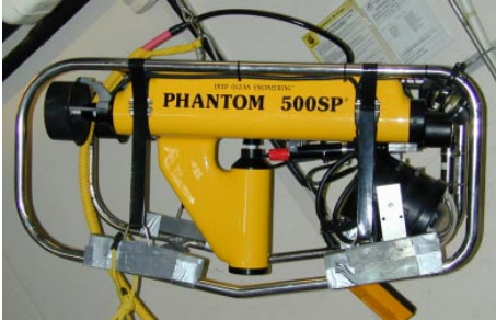
Fig. 4. Computer controlled Phantom ROV with the on-board camera. The camera housing is visible in the lower right, attached to the crash frame.
