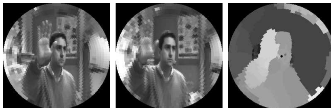
Fig. 3. The image in the right shows the raw foveated disparity map computed from the pair of images shown in the left, taken from a stereo head verging on a point midway between the foreground and background objects.
