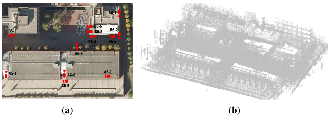
Figure 7. The Barcelona Robot Lab. (a) Aerial view of the camera distribution; and (b) the point cloud.
