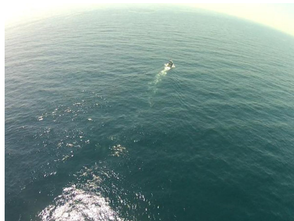
Figure 1. Vessel detection difficulties: moving camera, non stationary and dynamic background, sun reflections and sky.
