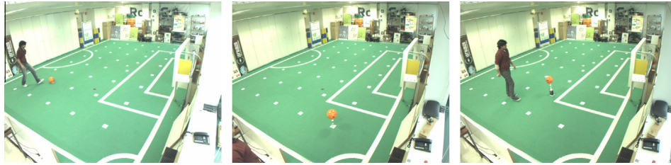
Fig. 6. Characterization of error within the ground truth (GT) estimation of the ball. Each of the above images show a different X, Y and Z coordinate placement of the ball from the right camera of the GT system at ISR, Lisbon. The origin of world-frame coordinates is at the center of the soccer field with positive X axis towards the yellow colored goal. (For interpretation of the references to color in this figure legend, the reader is referred to the web version of this article.)
