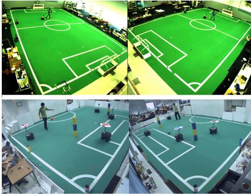
Fig. 5. Snapshot from the stereo vision system installed for ground-truth estimation of the robot's 2D and the ball's 3D positions. LSA lab facility of ISEP, Porto, Portugal (Top). Mobile Robotics Laboratory (LRM) at ISR, Lisbon, Portugal (Bottom).
