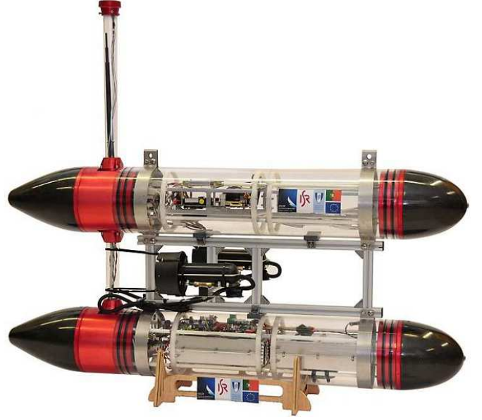
Fig. 2. The MEDUSA s surface craft. The thrusters are mounted in the middle between both hull parts on the x - z -plane (body coordinates) and produce completely from the body on the x - y -plane.
