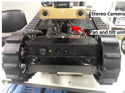
Figure 1.2: RAPOSA-NG with the stereo camera mounted on the Pan and Tilt Unit.
