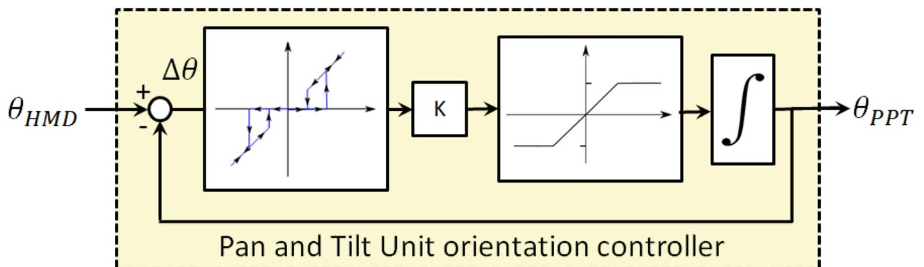
Figure 2.9: Physical pan and tilt controller
