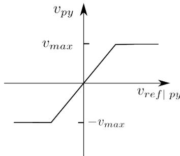
Figure 2.11: Saturation block transfer function.
