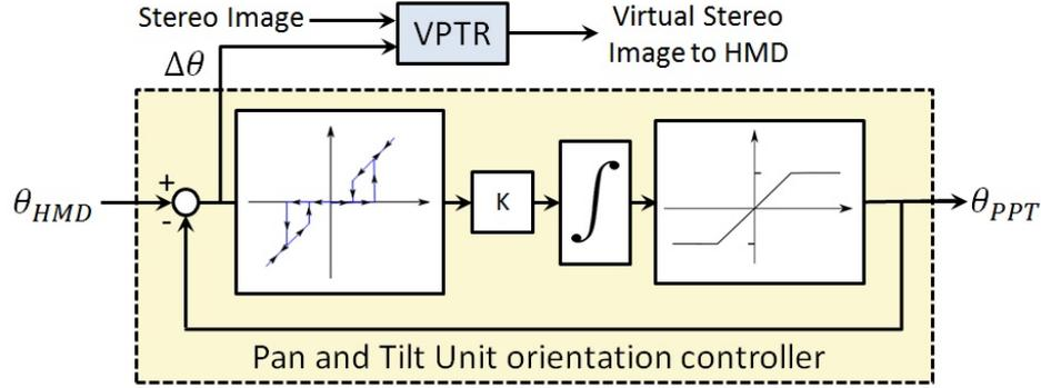
Figure 2.2: Block diagram of the controller.
