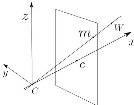
Figure 2.4: Pin Hole camera model
