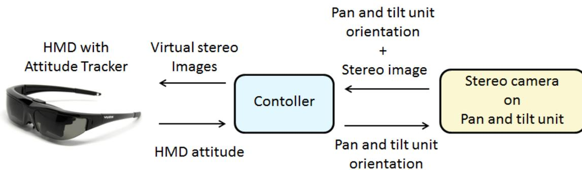
Figure 2.1: System Architecture with the Controller block
