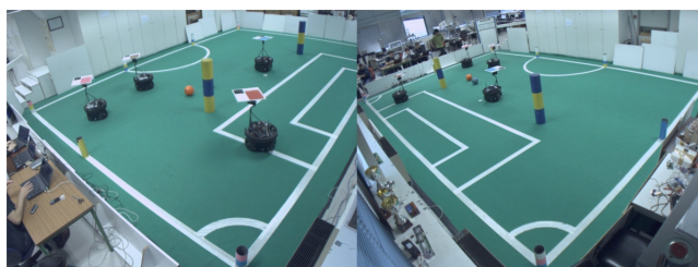
Figure B.1: Snapshot from the GTS installed for ground truth evaluation of the ball's 3D positions and the robots' 2D positions.
