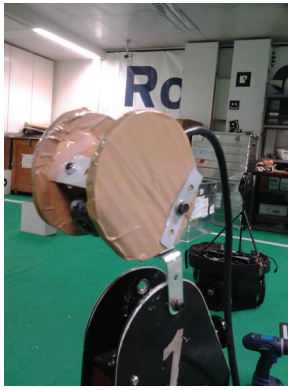
Fig. 2: Perspective lens-based camera mounted on top of a soccer robot
