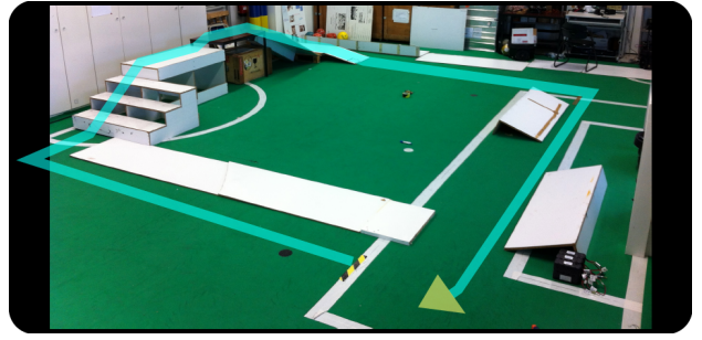
Fig. 4. Scenario used for experimental results. The indicated line represents the trajectory travelled by RAPOSA-NG during the experiment. The starting point is marked with black/yellow strips, and the path proceeds clockwise (with respect to the top view).
