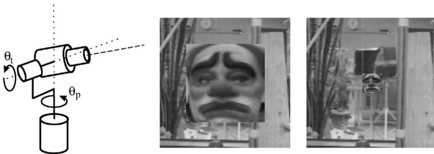
Fig. 7. Pan/tilt camera (left). The axis of rotation are assumed to intersect in the camera optical center. Simulated images with targets of scales 36% and 2.25% (right).
