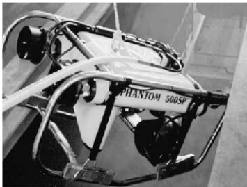
Fig. 3. Computer controlled Phantom ROV with an on-board pan and tilt camera.
