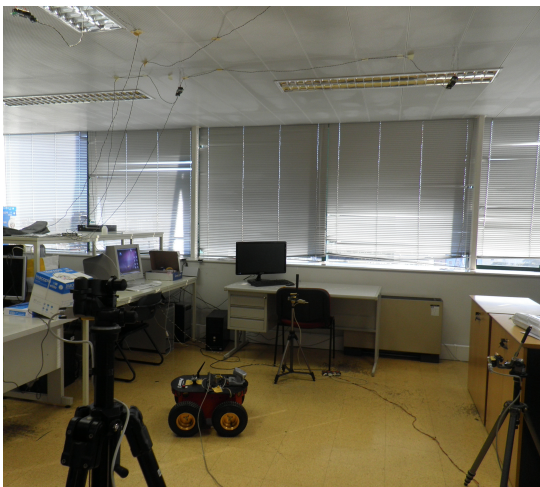
Fig. 1: The test environment and Pioneer P3-DX: 4 Cricket sensors on the ceiling and 4 on top of tripods distributed over the lab in a 4m x 4m area. The robot or a human carries the beacon.
