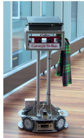
Figure 1: CoBot-2, an omnidirectional mobile robot for indoor users.
