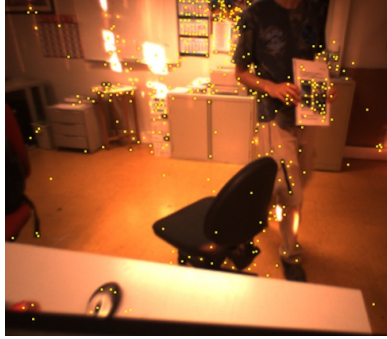
Fig. 3. Example of SIFT feature extraction; the dots (yellow) correspond to the extracted features positions.
