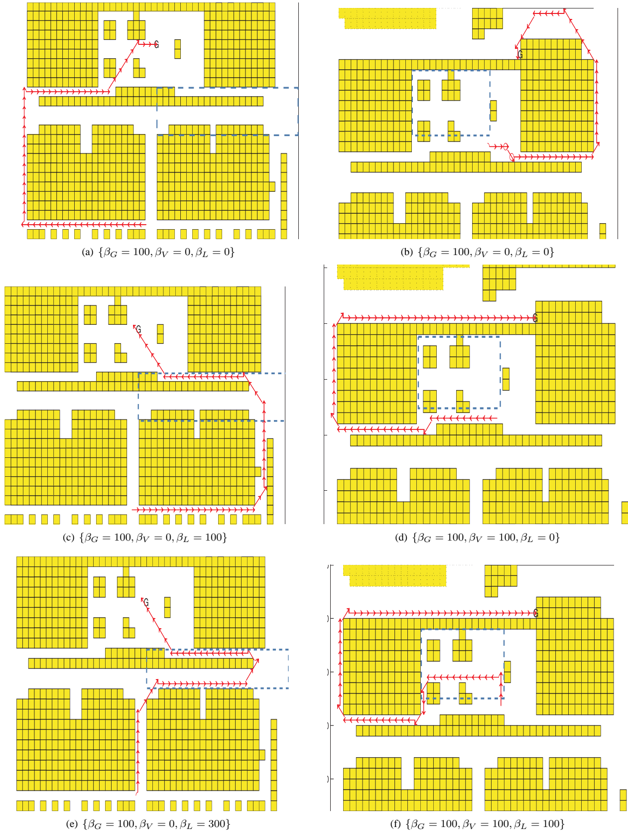
Fig. 4. The figures represents the generated path in different situations. In the figures, the dashed rectangle corresponds to a region covered by cameras, while the yellow squares are obstacles. To make the results better visible, only part of the scene shown in 3(b) in which the scenarios take place are shown. For all above cases, we set \beta_T = -1 and \beta_M = 0 .
