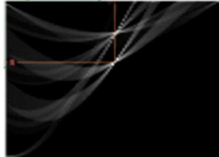
Fig. 10. Hough transform space. The horizontal coordinate is the straight line angle and the vertical one is the straight line distance to the origin.
