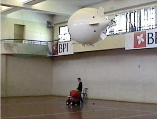
Fig. 15. Real blimp tracking a tele-operated iRobot ATRV-Jr robot.
