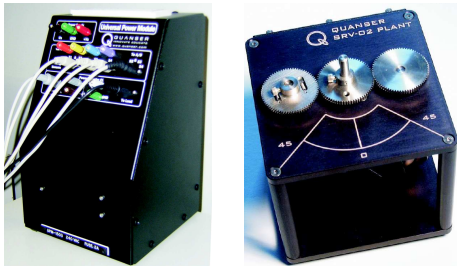
Figure 4: Power driver (left), the motor and sensors (right).
