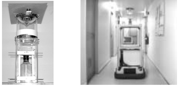
Figure 1: Left: the omnidirectional camera. Right: the camera mounted on the mobile robot.
