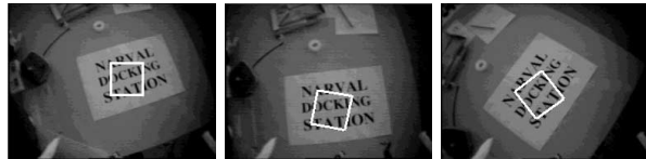
Figure 3: Tracking an image window from the flying blimp.
