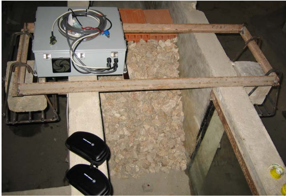
Figure 7. Laser mounted on the wave flume and rock slope to be surveyed.
