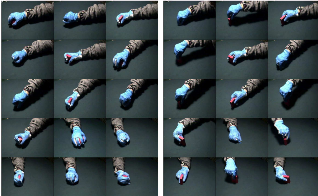
Figure 3.6: Data set illustrating some of the used grasp types: power (left) and precision (right). Altogether the tests were conducted using 60 sequences, from which a total of about 900 images were processed.
