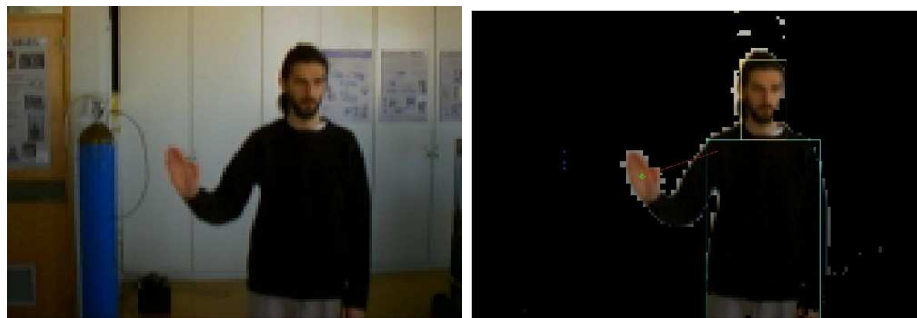
Figure 4.7: Vision system. Left: original image. Right: background segmentation with human (the rectangular frame corresponds to the template matching) and hand detection.
