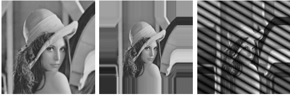
Fig. 6. Left: Original image. Middle: Image with boundaries extended by constancy. Right: Extended image modulated by a complex exponential with parameters \theta = 15 degree and \lambda = 29.6 pixel.
