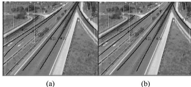
Fig. 9. (a) Final clustering result of lane center detection without using RANSAC estimation. (b) Final result using RANSAC estimation. Note that there is insufficient trajectory data to accurately represent the entry lane farthest from the camera.
