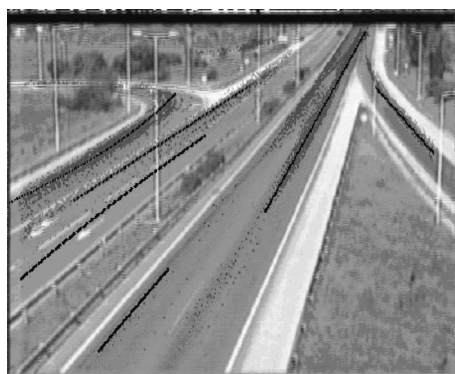
Fig. 8. Initialization of cluster means. Solid lines denote cluster centers and dots represent individual vehicle trajectories.
