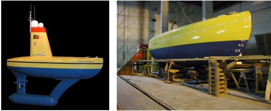
Figure 5. The Caravela autonomous research vessel. Left: a scale model; Right: the vehicle hull in the shipyard.
