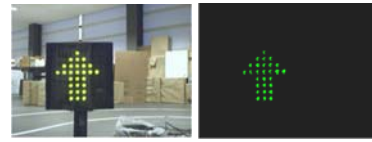
Fig. 9 – Sign segmentation by saturation and hue analysis
