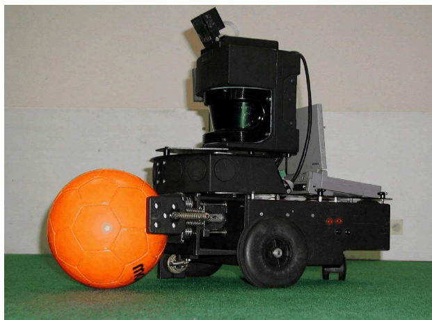
Figure 7: CS Freiburg player mounting SICK LRF, color camera, Libretto laptop, WaveLan wireless ethernet and custom-made new kicking device.
