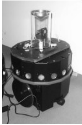
Fig. 2. Catadioptric system assembled on the robot.
