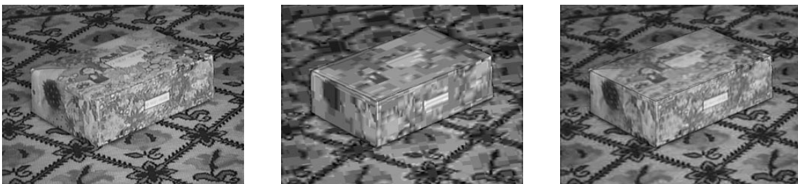
Figure 11.5: Video compression. Left: frame 1 of the box video sequence, Center: frame 1 of the synthesized sequence for a compression ratio of 575:1, Center: frame 1 of the synthesized sequence coded for a compression ratio of 317:1.
