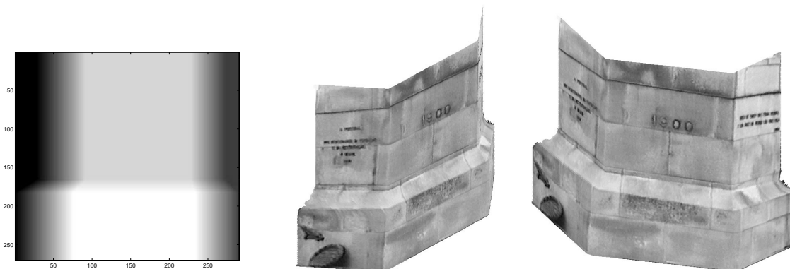
Figure 11.7: Relative depth and reconstructed 3D shape and texture for the pedestal video sequence of Figure 11.6.
