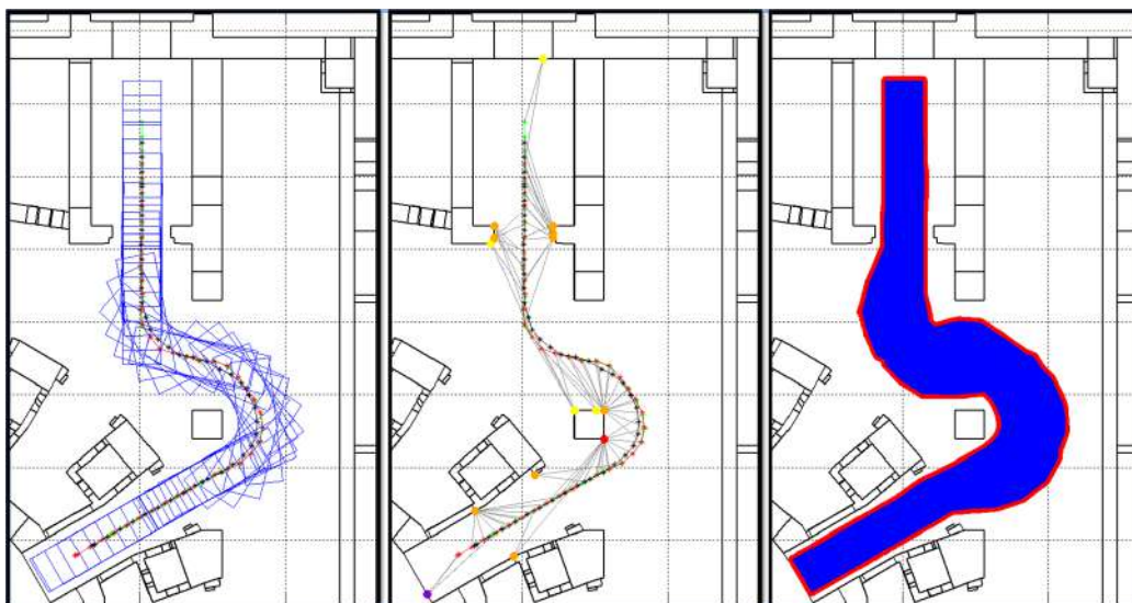
Figure 16: Trajectory to port 2 using line guidance (from left to right), path and sampling poses, the most closest obstacles and the area spanned by the vehicle along the path.
